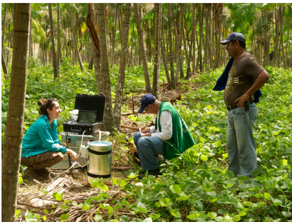
Soil respiration determination in an Acai plantation (Loc 07) with Laura Medeiros Braga, Gilvan Coimbra Martins and Edinilson Alves Figueiredo (f.l.t.r.), phase 1 of the project
