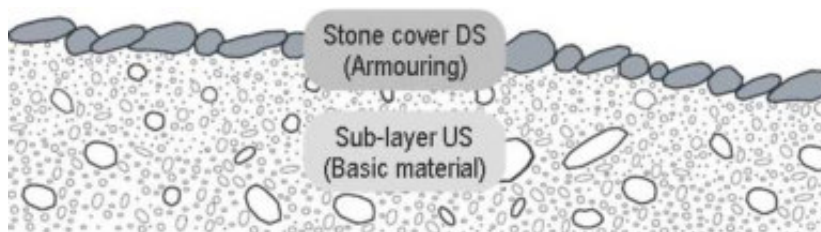
Fig. 2.16: Stone cover and sub-layer at river ground (after BEZZOLA, 2004)
