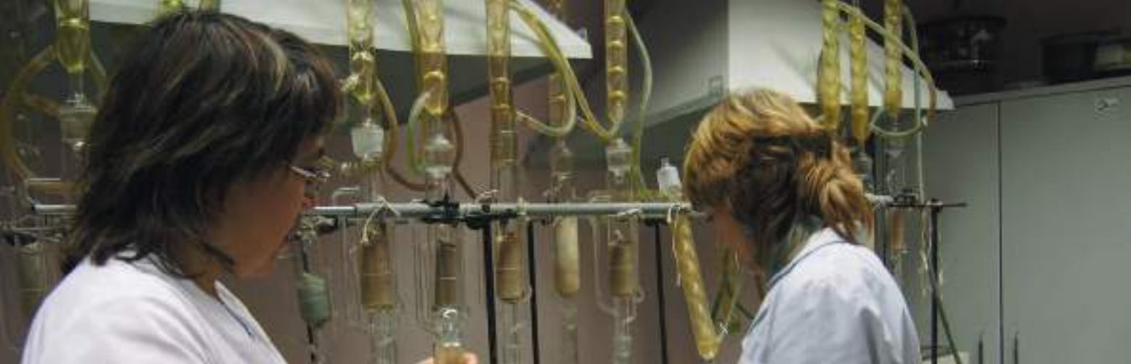
Extraction of oil from the core samples
