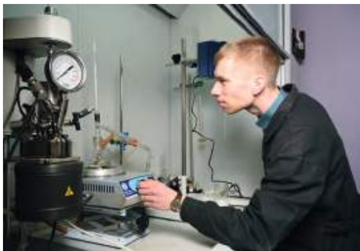
Digestion bomb Parr Instruments
