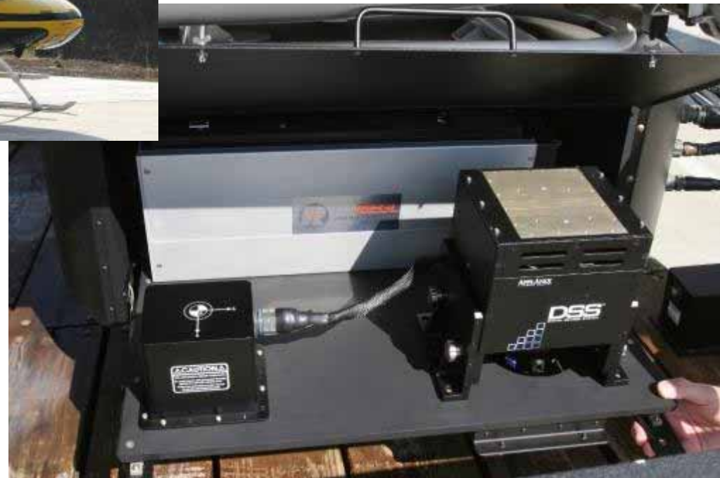
Custom Integration RIEGL Q560 – Bell Jet Ranger
